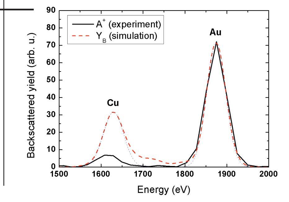
scattered from CuAu(001) - [110] azimuth. Au and Cu can be separated easily.
